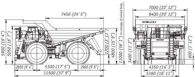
\*Overall dimensions are specified for basic kitting-up of the dump truck
